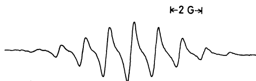
Fig. 1. ESR spectrum of 3.0 \times 10^{-4} \text{ M} TCNE-Cs + in THF at 25 °C.
